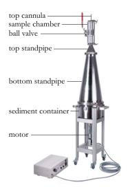
Fig. 1 Components of the MPSS. Photo by Hydro-Bios Apparatebau GmbH, modified
